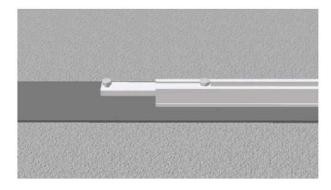
The mounting rails must be positioned with the wide side downwards onto the protective mat, so that the mean distance amounts 800 mm. When connecting several collectors, the mounting rails must be connected as well. The screws fix the brackets at the same time.
