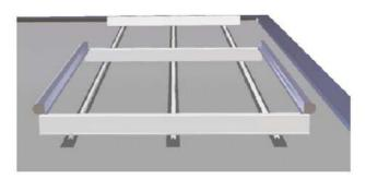
The mounting rails must be connected with help of the rail connectors with the mounting rails as well. The screws also fix the supporting brackets.
