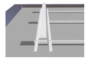
When mounting the supporting brackets, the hexagon screws M8 of the connector must be screwed into the designated holes, but must not be tightened yet. The supporting brackets must be placed within the connection point.
