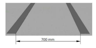
The protective mat ensures through its special characteristics slip resistance of the mounting rails and protects the roofing. The distance between the stripes amounts 700 mm.
