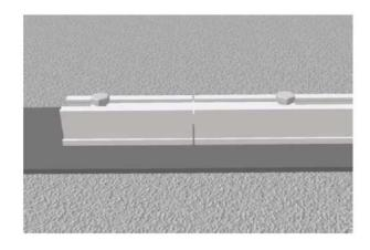
The end-pieces of the mounting rails must be connected with help of the rail connectors with the mounting rails. The screws also fix the supporting brackets.
