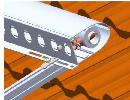
Installation of the manifold
