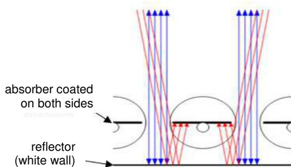
At the normal irradiation, most of the light is directly reflected from the reflector and light does not reach the lower absorber surface area.
