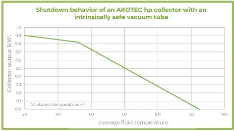
Tube collector output with solar radiation of 1,000 W/m<sup>2</sup> (collector with 10 tubes)
